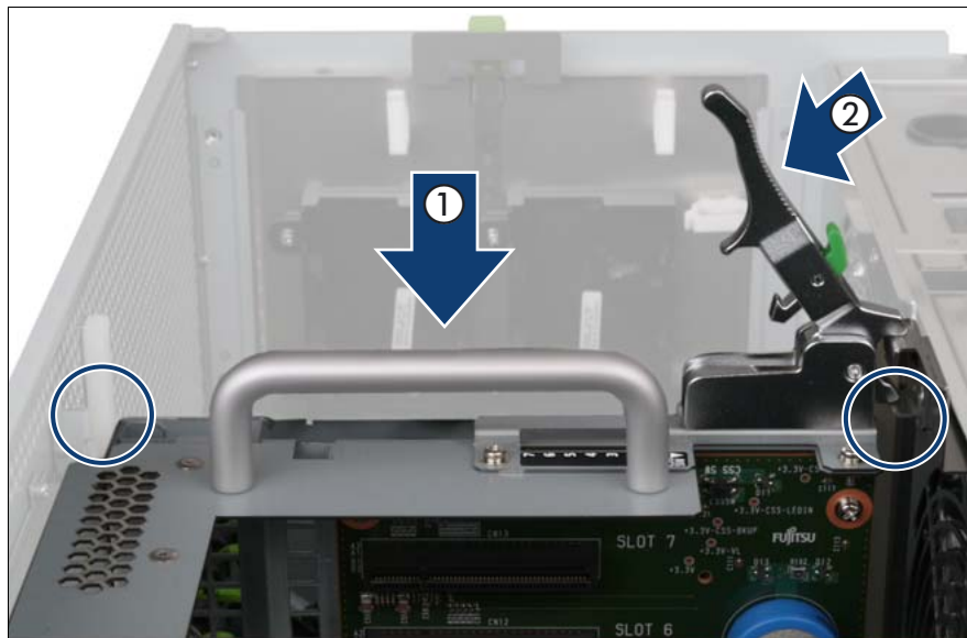
Figure 98: Installing the PCI Riser
